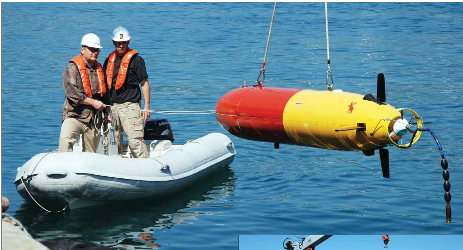
Two scientists from the NATO Undersea Research Centre in La Spezia, about an hour north of Camp Darby, lower an Autonomous Underwater Vehicle into the La Spezia bay in order to test its radar capabilities.
