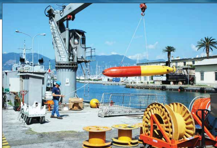
A scientist prepares to lower an Autonomous Underwater Vehicle into the La Spezia bay. The AUV is part of the NATO Undersea Research Centre's efforts to develop underwater technology.
